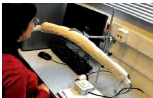
Fig. 2 96 temperature modulated chemical sensor array to test redundancy and diversity coding in the olfactory system.
