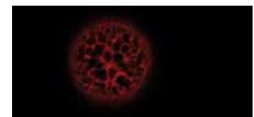
Fig. 2 (right) Confocal image of a PLGA microparticle of 60 µm.
