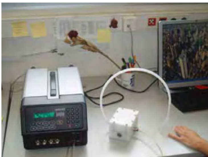
Experiments using a mechanical ventilator to investigate on the influence of breathing dynamics on the response of artificial olfaction systems.
