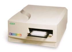
The Bechmark Plus microplate reader from Bio-Rad can be used for **absorbance assays**. It has the capability to perform standard colorimetric ELISA and kinetic readings for general cell screening with 6, 12, 24, 96, and 384-well microplate formats. The microplate reader uses a xenon flash lamp as light source and has a "filter-less" design, with a wavelength range of 340-800 nm, which allows the user to set the
