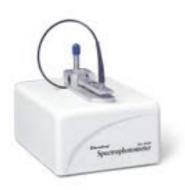
The Nanodrop ND-1000 is a full-spectrum (220-750 nm) spectrophotometer that measures 1  $\mu$ l samples with high accuracy and reproducibility.
