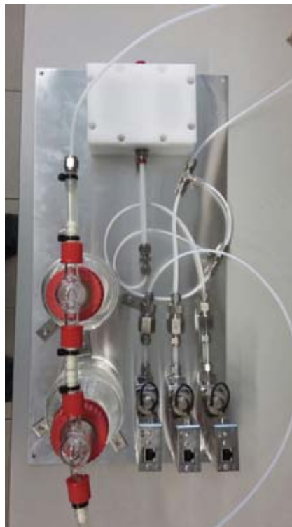
System to test chemical sensors for malodour detection
