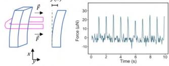
3D-bioprinted bio-actuator based on skeletal muscle used as a force measurement platform. Upon electrical stimulation, the muscle can contract, bend the post and their force can be calculated.
