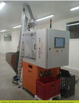
Fast TCA detection in corks using lon Mobility Spectrometry technology (in collaboration with 3control Industrial Automation and Vision SL).
