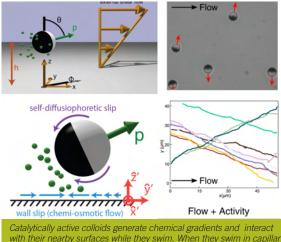
enhance chemical reactions while they swim. These micromotors are mostly based on two main structures, tubular and spherical.
