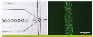
Microfluid chip for droplet generation and encapsulation.
