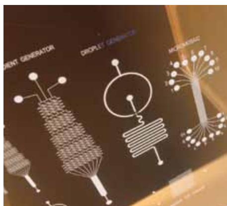
Photomask with distinct microfluidic designs such a gradient generator, a droplet generator or a fluidic system for immunoassays
