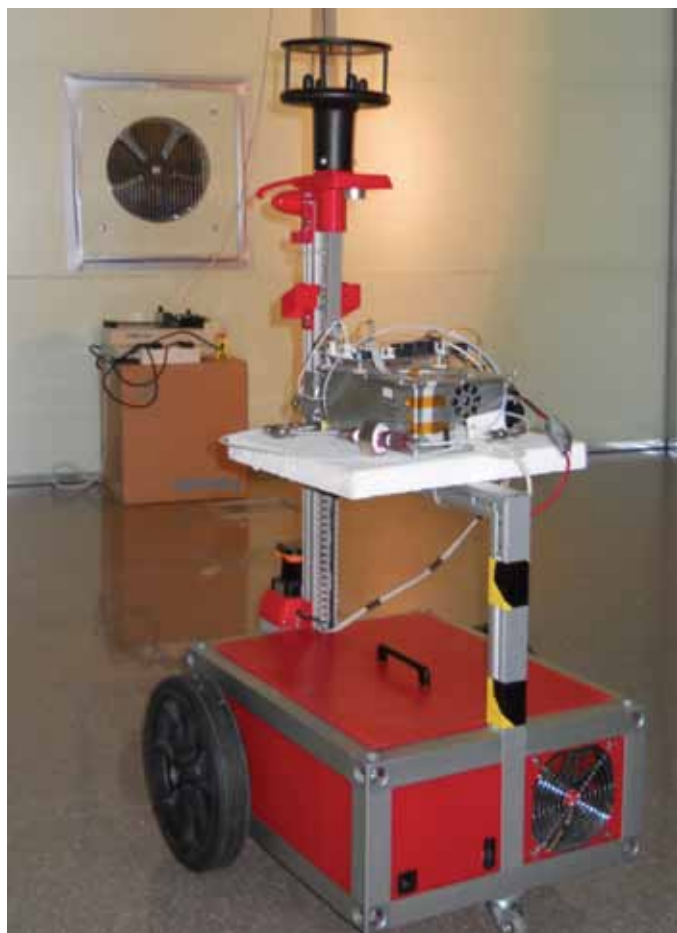
Autonomous Robot fitted with a Field Asymmetric Ion Mobility Spectrometer for Chemical Source localization experiments.
