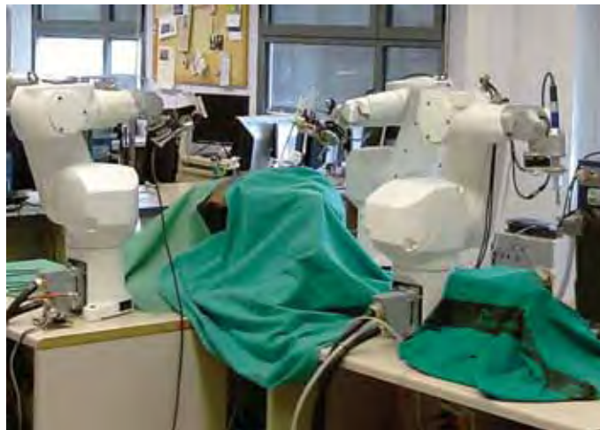
Experimental surgical robot platform for laparoscopic surgery (with CREB-UPC).
