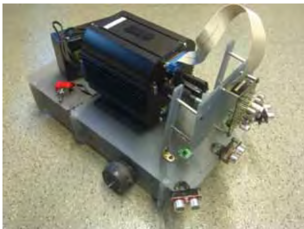
Neuromorphic Odor robot including chemical sensor arrays and embedded computational models of the insect olfactory system developed in the NEUROCHEM project (joint development with UPC and UPF)
