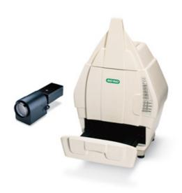
Gel Doc XR+ imaging system is a highresolution gel documentation system that allows fast, easy quantitation of gels and blots. It uses a CCD camera to capture images in real time.
