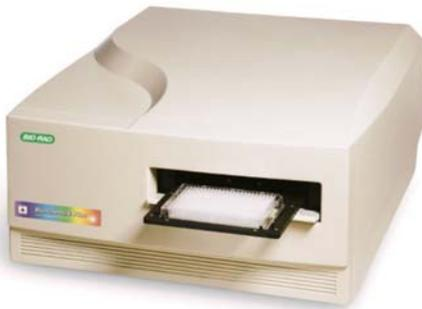
The Benchmark Plus microplate reader from Bio-Rad can be used for **absorbance assays**. It has the capability to perform standard colorimetric ELISA and kinetic readings for general cell screening with 6, 12, 24, 96, and 384-well microplate formats. The microplate reader uses a xenon flash lamp as light source and has a “filter-less” design, with a wavelength range of 340-800 nm, which allows the user to set the
