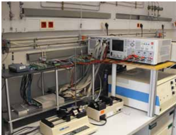
System to test chemical sensor arrays for diversity and redundancy
