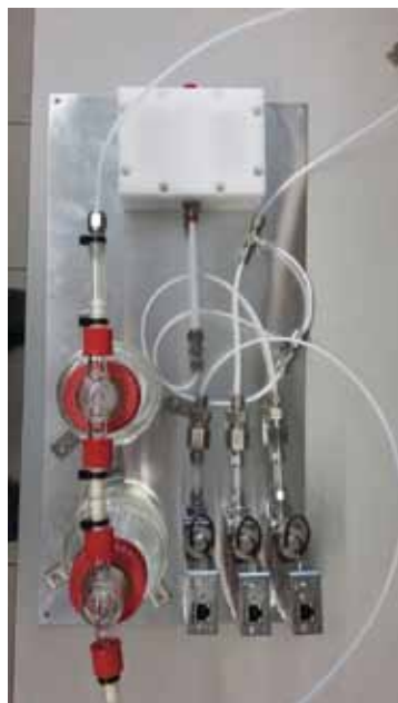
System to test chemical sensors for malodour detection
