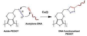
**Fig. 1.** Construction of PEDOT-based DNA sensor: DNA immobilization process by "click" reaction, using Cu(I) source.
