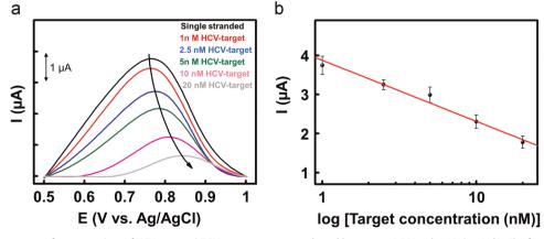
Fig. 5. Sensor response to a range of concentrations of HCV-target. a) DPV measurements, conducted between +0.5 V and +1 V (vs. Ag/AgCl reference electrode) at 100 mV/s in 20 mM Tris-HCl buffer at room temperature and b) corresponding calibration curve, where current intensity is plotted against the logarithm of HCV-target concentration. Error bars are the standard deviation of three independent experiments.
