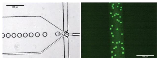
Microfluidic chip for droplet generation and encapsulation.
