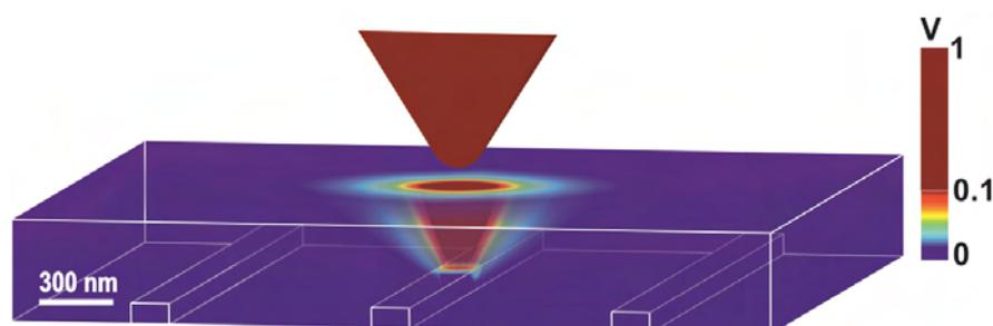
Voltage distribution numerically calculated for a nanochannel-electrostatic force microscope tip structure. The numerical calculations have been used to quantify the electrostatic force acting on the tip as a function of the thickness of the nanochannels containing water. These calculations allowed demonstrating an anomalously low dielectric constant of water confined in nanochannels. The height of the channels varied from 1 nm to 200 nm and they are buried below a layer 50 nm thick.
