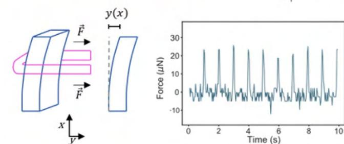
3D-bioprinted bio-actuator based on skeletal muscle used as a force measurement platform. Upon electrical stimulation, the muscle can contract, bend the post and their force can be calculated.
