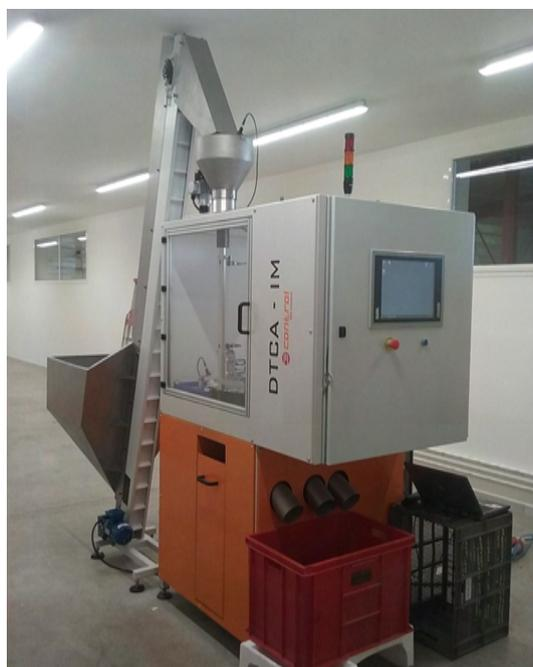
Fast TCA detection in corks using Ion Mobility Spectrometry technology (in collaboration with 3control Industrial Automation and Vision SL).
