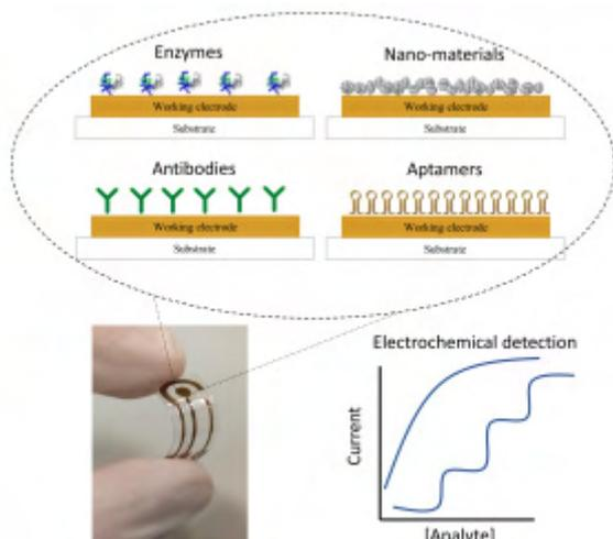
Electrodes fabricated on flexible substrates are modified with a wide range of materials for selectivity towards biomarkers. Analytes are quickly quantified by electrochemical techniques.
