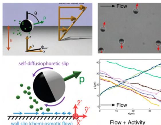
Catalytically active colloids generate chemical gradients and interact with their nearby surfaces while they swim. When they swim in capillaries where a flow is imposed, they present a cross stream migration deviating from straight trajectories, perpendicular to the flow lines. This type of motion resembles, in some aspects, the motion of biological microswimmers.
