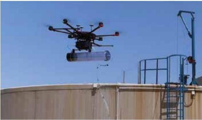
The company Depuración de Aguas del Mediterráneo (DAM) and the Institute for Bioengineering of Catalonia (IBEC) develop a system equipped with chemical sensors that provides information, in real time, on the intensity and location of odor sources in the Waste Water Treatment Plants (WWTP). The system has been calibrated and validated under real operating conditions through several measurement campaigns at the Molina de Segura WWTP (Murcia).
