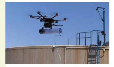
The company Depuración de Aguas del Mediterráneo (DAM) and the Institute for Bioengineering of Catalonia (IBEC) develop a system equipped with chemical sensors that provides information, in real time, on the intensity and location of odor sources in the Waste Water Treatment Plants (WWTP). The system has been calibrated and validated under real operating conditions through several measurement campaigns at the Molina de Segura WWTP (Murcia).
