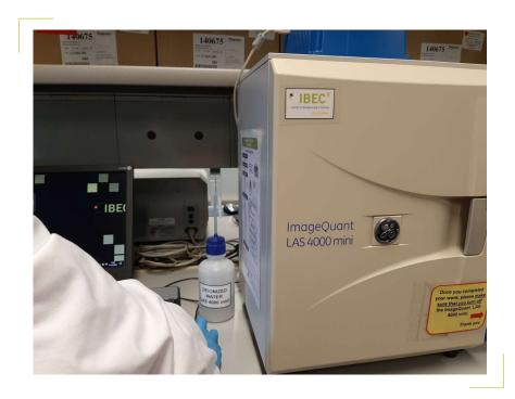
ImageQuant LAS 4000 mini is a dedicated CCD camera system for sensitive, quantitative imaging of gels and blots by chemiluminescence and white epi-illumination gel documentation. The system bought by IBEC also has a blue epi-fluorescence module.
