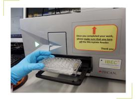
The Infinite M200 PRO from Tecan can provide a full range of leading detection methods. The Quad4 Monochromators of the Infinite M200 PRO provides exceptional sensitivity and allows the user to select any wavelength from UV to NIR, and to perform absorbance, excitation and emission scans. Users can access all wavelengths, and change from top to bottom reading, for easy measurement of multiplexed assays.
