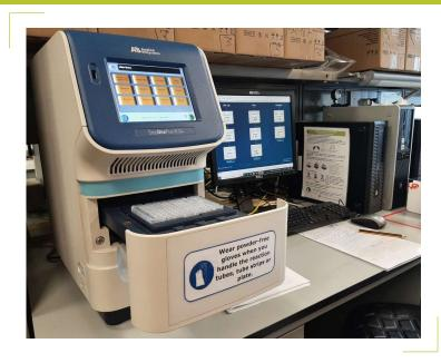
The StepOnePlus System from Applied Biosystems supports any real-time PCR application, such as:
