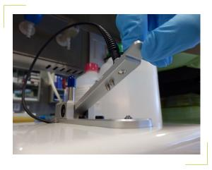
The Nanodrop ND-1000 is a full-spectrum (220-750 nm) spectrophotometer that measures 1  $\mu$ l samples with high accuracy and reproducibility.
