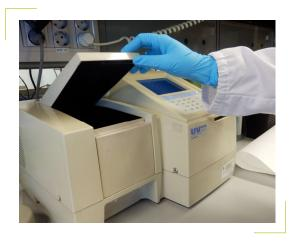
The UVmini-1240 is an ultraviolet visible spectrophotometer.
