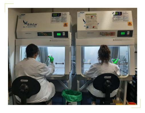
The Biospace has several BIO-II A cell culture cabinets for working with biosafety levels 1 and 2 cell cultures.
