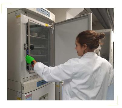
CO2 Incubators with water jacket technology that protects the cell cultures against ambient temperature swings and HEPA filters that provide clean room quality air purity, minimizing the risk of airborne contaminants.
