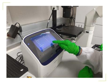
The Invitrogen Countess 3 is an automated cell counter that utilize a machine-learning algorithm to analyse trypan blue stained samples in suspension and generate highly accurate cell counts.
