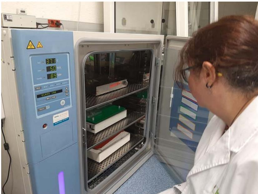
The Gadget Incubator is the largest capacity CO<sub>2</sub> incubator available at the facility and features an active humidification system, HEPA filters and IR CO<sub>2</sub> sensor for optimum cell viability.
