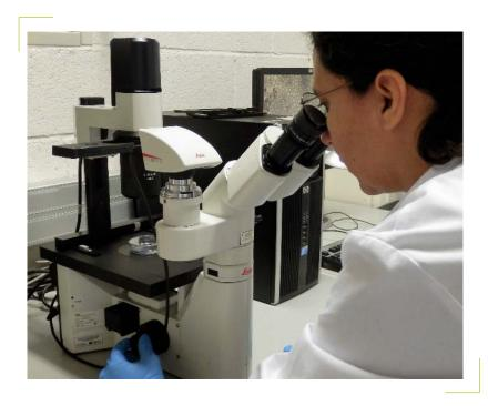
The Leica DMIL LED is versatile inverted fluorescence microscope equipped with a Leica MC190 HD camera and workstation.
