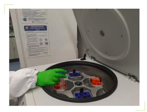
The 5810 R is a refrigerated bench-top centrifuge equipped with a A-4 62 rotor with adapters for 15-and 50-ml conical tubes and cell culture plates.
