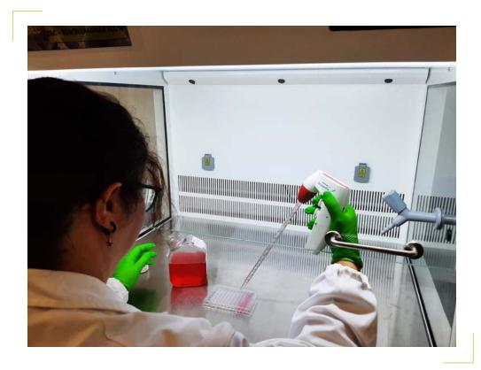
The Biospace has a vertical Laminar Flow cabinet that allow to work with non dangerous materials in a dust-free and sterile environment.
