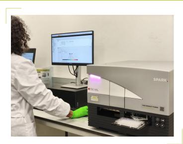
Our Multimode Microplate Reader – SPARK – offers a comprehensive range of advanced detection methods. Equipped with Quad4 Monochromators, the Spark multimode reader delivers exceptional sensitivity, enabling users to select any wavelength from UV to NIR and perform absorbance, excitation and emission scans.
