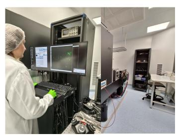
Vertical multiphoton microscope for the stimulation and obtaining of intravital fluorescence images.
